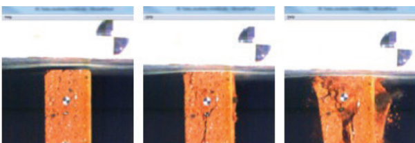
High Speed Video sequence for brick under dynamic compression test.
