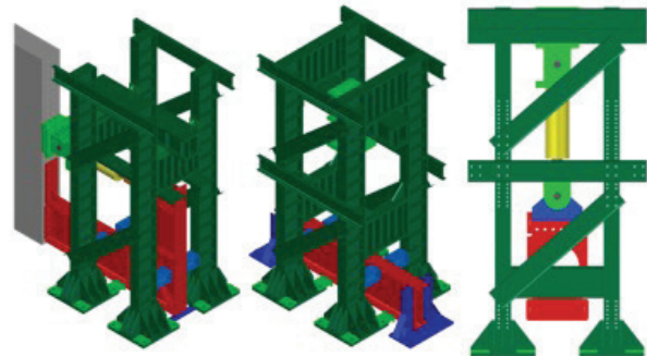
Schematic representation of the defined test set-up for the LBNF steel joints
