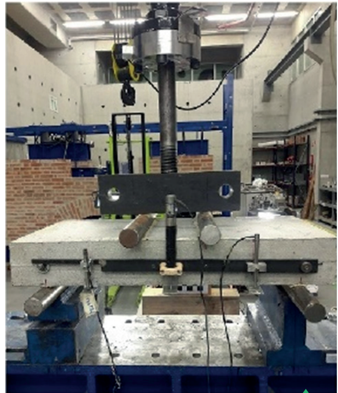
Flexural behavior of plates made by HPFRSCC and reinforced with 3D-SRT
