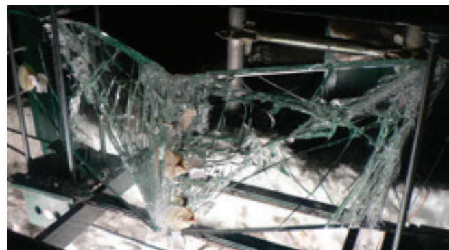
Test with temperature load: Fracture pattern
