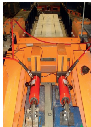
(a) Prestressing a RC slab
