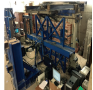
(a) Testing setup for tie-masonry connections; (b) Testing setup for Brick veneer walls under out-of-plane loading
