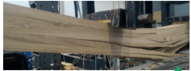
Failure mode of Eucalyptus beam – punctual propagation of failure along the glue line 2
