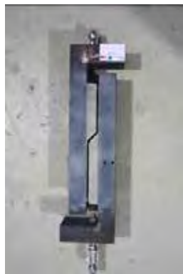
Fig. 1 Shear tests performed in the foam core material – shear failure mode (Task 4)
