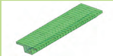
FEM model of the bridge
