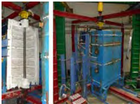
Fig. 2 Experimental set-up for CFS columns
