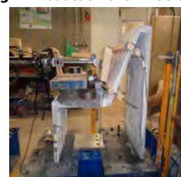
Fig. 3 Chair in FRCC being tested
