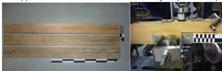
Fig. 3 Experimental campaign using acoustic emission for crack evolution assessment (Task 2, 3)
