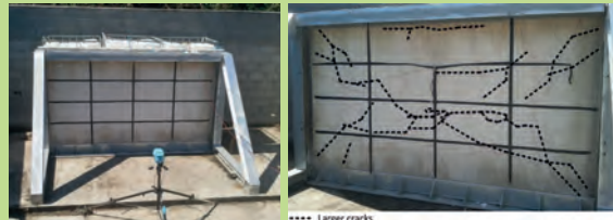
Out-of-plane setup for walls under blast loading
