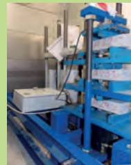
Fig. 6 Creep flexural test
