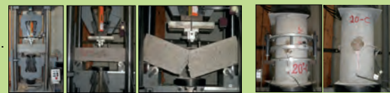
Fig.4 Test set-up for the residual flexural tensile strength tests.
