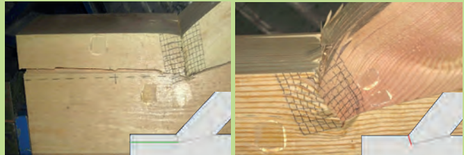
Figures 1 and 2: Failure modes in the Single Step Joint – Shear crack in the tie beam (left), crushing at the front-notch surface (right).
