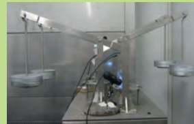
Fig. 4 Fibre pull-out creep test
