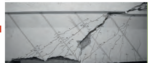
Fig. 1a-c : result of the proposed model (PDS model) Versus the test observations for the beam 3S-4LI-S2
