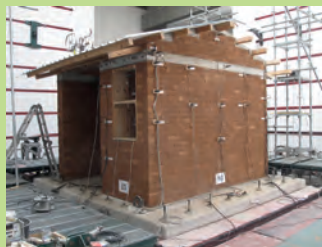
Fig. 7 - Shaking table test of small masonry house: (a) mock-up; (b) envelopes.
