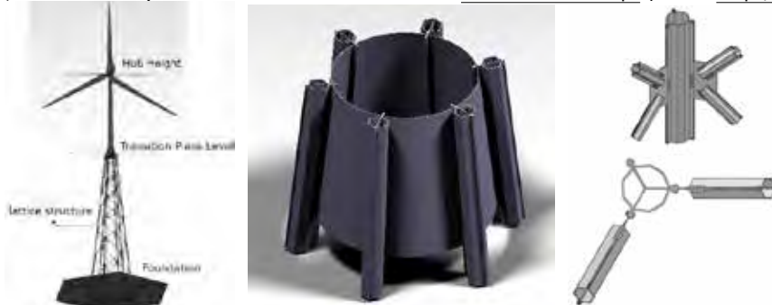
Fig. 1 Hybrid Tower concept with components
