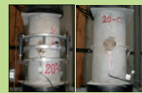
Fig.5 Test set-up for the residual modulus of elasticity and Poisson's ratio tests.
