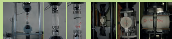
Fig.2 Test set-up for the residual direct tensile strength tests.
