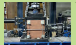
Fig. 5 - Triplet shear test: (a) test setup; (b) compression vs. shear strength.
