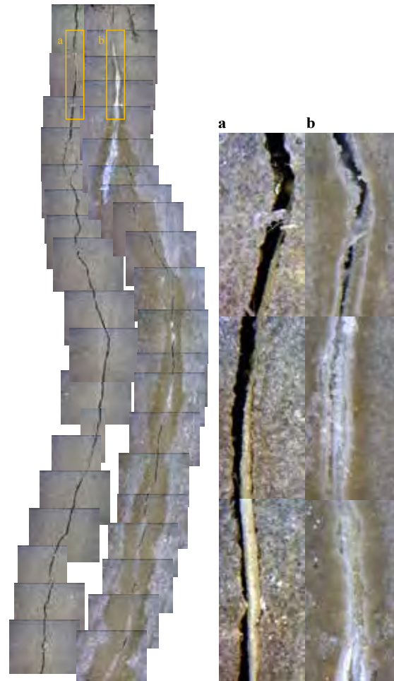
Fig. 4 Effect of natural water exposure time on recovery of composite: Crack before (left-a) and after 1 month in water (left-b): Sisal + Steel specimen; Magnification on 200x (Right-a, b)
