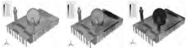
Fig. 9 Al-Askari holy shrine - deformed mesh evolution due to external explosion close to the structure
