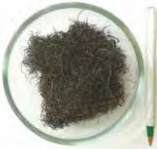
Fig. 2 A sample of recycled steel fibers
