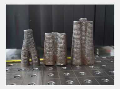
The CMT welding process allows for welding at much lower temperatures and therefore reduce the possibility of distortions and imperfections in the final product. The system range covers an area of about 5 x 3 meters.
