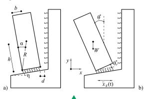
Distinct element model of masonry specimen. a) Configuration before each test: initial out-of-plumb? and gap d related to mortar vertical joint. b) Kinematic descriptors of the motion: out-of-plane rotation of the faÁade wall measured with respect to the vertical (?) and to the titled foundation (?r).
