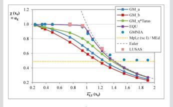
Improvement of the proposed methodology in comparison to other possible methodologies and current approaches for tapered beams.
