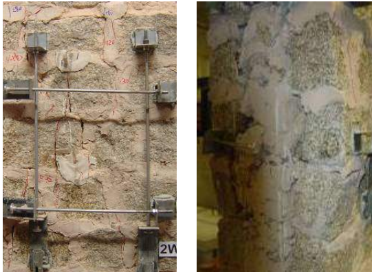
Figure 5 – Observed failure modes (transversal tying).
