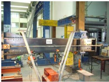
Fig 5 – Experimental test of the connection column-foundation.
