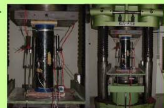
Test of a strengthened column
