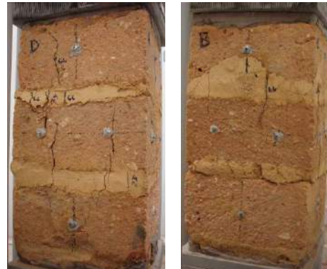
Figure 8 – Typical crack pattern during testing (adobe prism).
