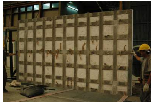
Fig. 11 - 4.100x2.200x0.11 m³ SFRSCC lightweight panel.
