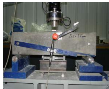
Fig. 3 – Bending Test according to RILEM TC 162-TDF.
