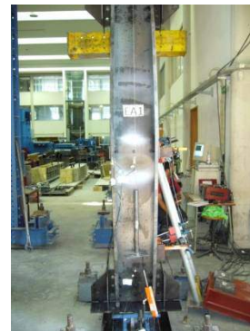
Fig 2 - A compression test with two C profiles gathered by the web in a discontinuous way.
