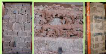
Unstrengthened wall tested under compression
