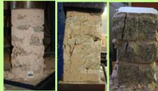
Three-leaf wall components: plain inner core, injected core and external leaf.
