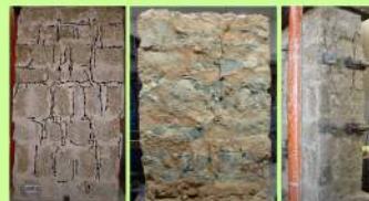
Injected wall tested under compression
