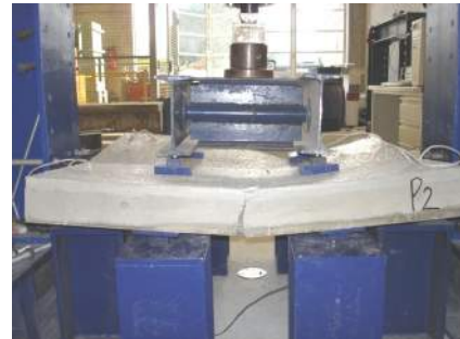
Fig. 9 - Bending Test in Panel Prototypes.
