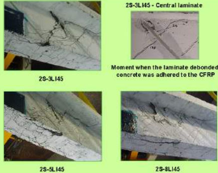
Note: the differences between the tested beams were restricted to the shear reinforcement systems applied in the smaller shear span.
