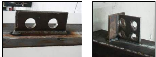
Fig 1 - Perfbond and T-Perfbond connectors being developed by the Portuguese and Brazilian Teams
