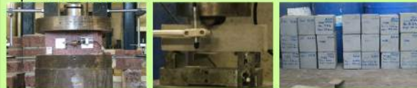
Figure 5 – Evaluation of mechanical properties of materials: masonry units, mortar and concrete infill.
