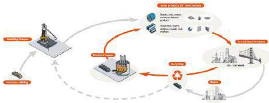
Fig. 1 Life cycle of steel structures.
