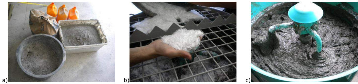
Fig. 1 SHCC composition. a) components; b) glass fibers; c) final aspect.
