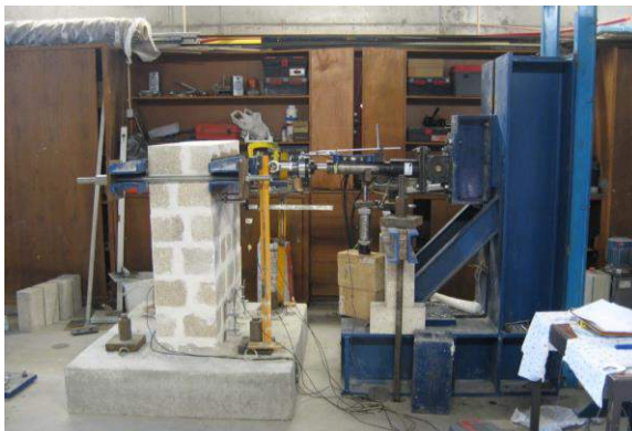
Fig. 2 Application of the improved technique with heli-needles.
