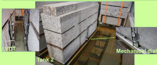
Monitoring of mid-span deformation during creep tests
