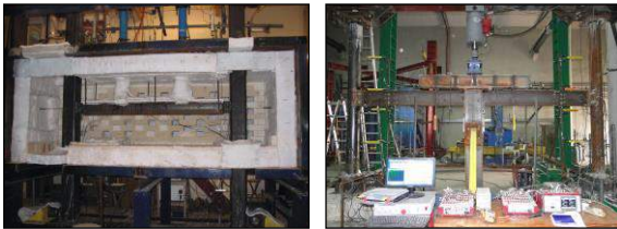
Fig. 2 Testing schemes proposed to experimental fire testing of structural subassemblies (small- and full-scale tests).
