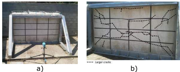
Fig. 5 Structural element testing: a) out-of-plane setup for walls under blast loading; b) URM wall under WBWG loading.
