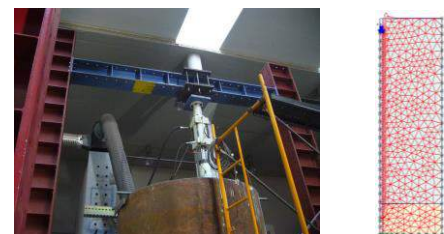
Fig. 3 Experimental small-scaled micropile load tests and numerical evaluation.
