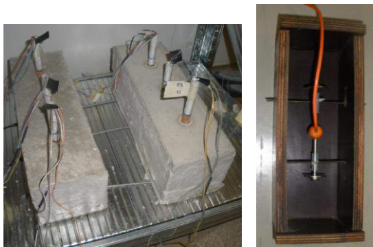
Fig. 3 Concrete specimens with embedded humidity sensors; embedded strain gages in formwork for shrinkage monitoring
