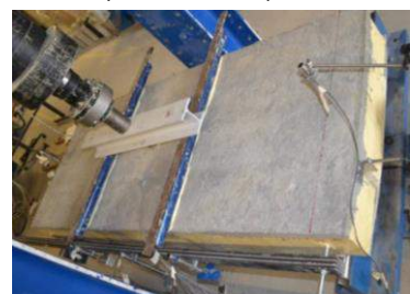
Fig. 3 Assessment of hybrid slabs under static four point bending test.
