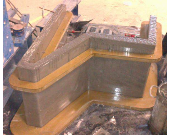
Fig. 2 Acrylic mould used during the casting process of a chair.
