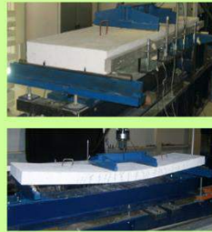
Four point bending test
