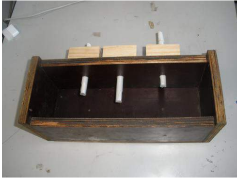
Fig. 1 Formwork with pre-placed tubes for humidity measurement.
