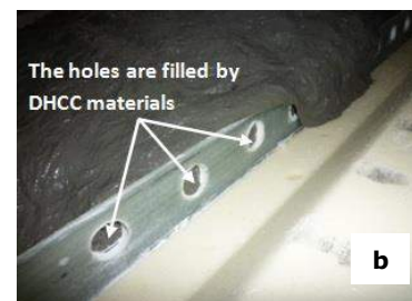
Fig. 2 Manufacture process of hybrid slabs: a) VARTM process; b) Casting of DHCC materials.
