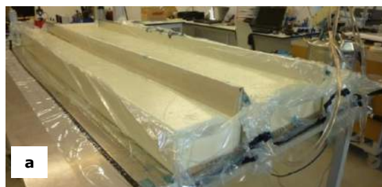
Fig. 2 Manufacture process of hybrid slabs: a) VARTM process; b) Casting of DHCC materials.
