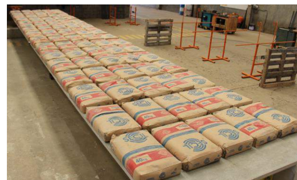
Fig. 8 Structure loaded for the creep test.
