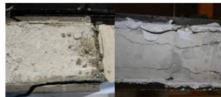
Fig. 2 Debonding of the HCPs.
