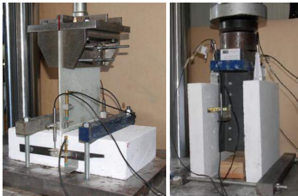
Fig. 4 Experimental tests on GFRP shear connection.
