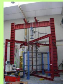
1. 3D restraining steel frame; 2. Hydraulic jack of 3MN; 3. Load cell (LC); 4. 2D reaction frame; 5. safety structure; 6. LVDT's; 7. Cable LVDT's; 8. Modular electric furnace; 9. Special device with LC;
