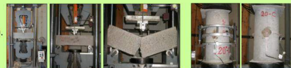
Fig.4 Test set-up for the residual flexural tensile strength tests.
