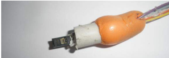
Fig. 2 Humidity sensors for embedment in concrete: mounting devised in the scope of the research project.
