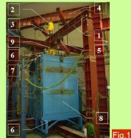
1. 3D restraining steel frame; 2. Hydraulic jack of 3MN; 3. Load cell (LC); 4. 2D reaction frame; 5. safety structure; 6. LVDT's; 7. Cable LVDT's; 8. Modular electric furnace; 9. Special device with LC;
