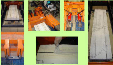
Application of prestress in RC slabs
