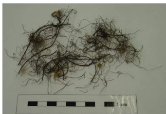
Fig. 1 Recycled steel fibers extracted from rubber tyres.
