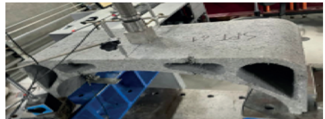
Testing an FRC block, a component of the developed lightweight slab
