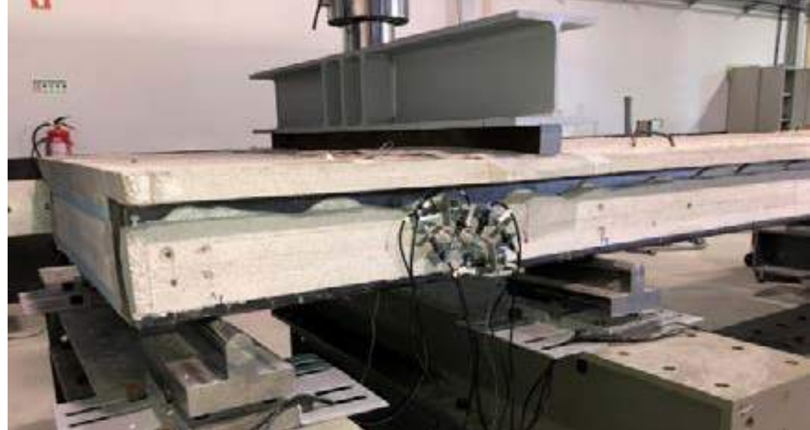
Photographs of PreSlabTec prototypes tested in: bending (left), and shear (right).
