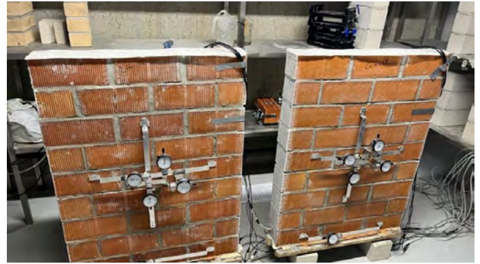
Examples of the wallettes for moisture expansion test
