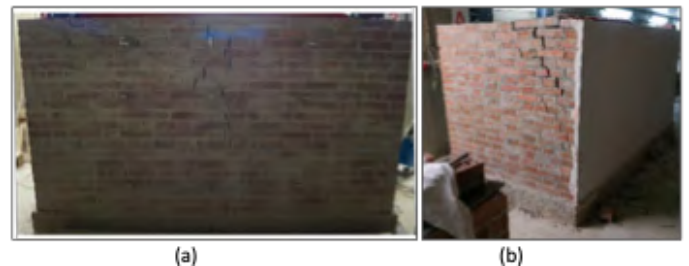
Post airbag test damage pattern in (a) UMW façade (b) RMW right side
