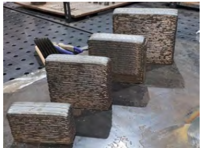
WAAM carbon steel material produced at ISISE AMConstruction Lab
