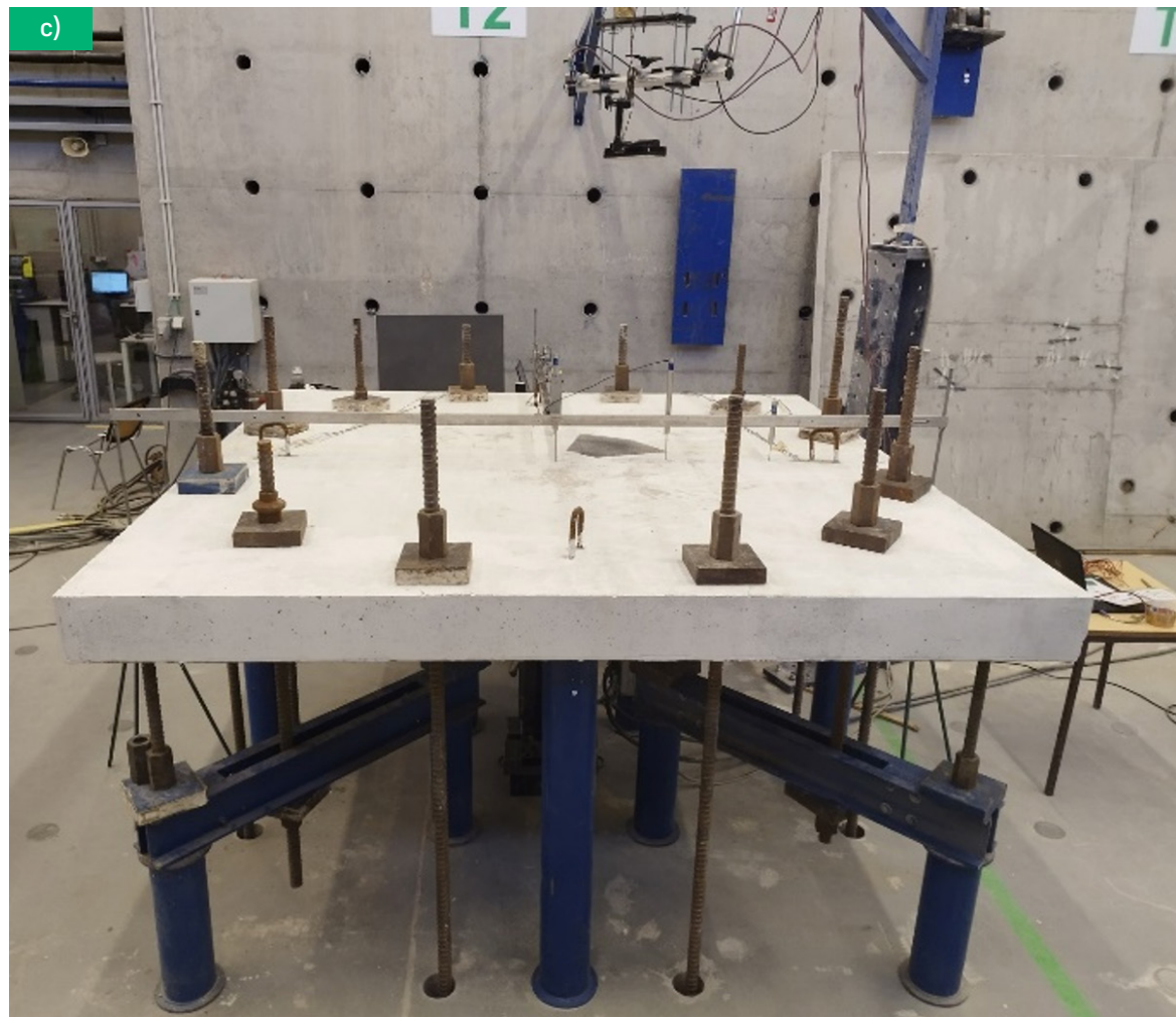
Fig. 1 – Blind simulation competitions executed: a) 1st – FRC T cross section beams failing in shear; b) 2nd – FRC shallow beams failing in bending; c) 4rd – FRC prototypes of slabs failing in punching.
