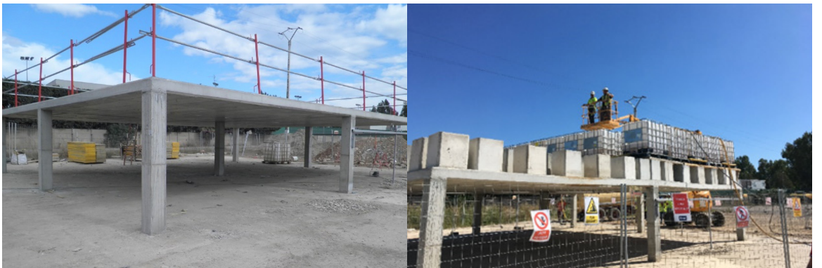
Fig. 3 – Full-scale test used to assess the predictive capability of global resistance methods applied to FRC slabs supported on columns.
